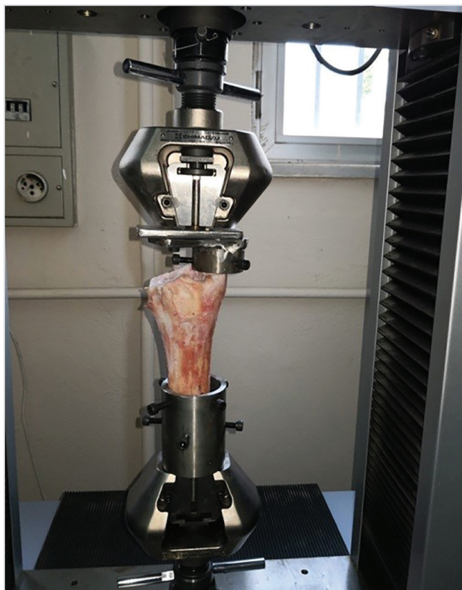
Figure 2. Application of tensile forces to the prepared samples
