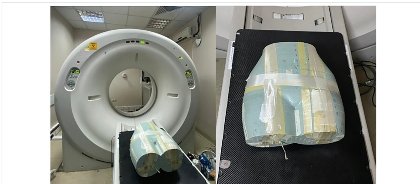
Figure 3. Positioning of the CIRS female pelvic anthropomorphic phantom on the Toshiba Aquilion 64-slice CT scanner. The phantom was placed in the supine position and aligned at the scanner isocenter using the built-in laser positioning system to ensure reproducible imaging geometry during abdominal–pelvic CT acquisitions. CIRS: Computerized Imaging Reference System, CT: Computed tomography
