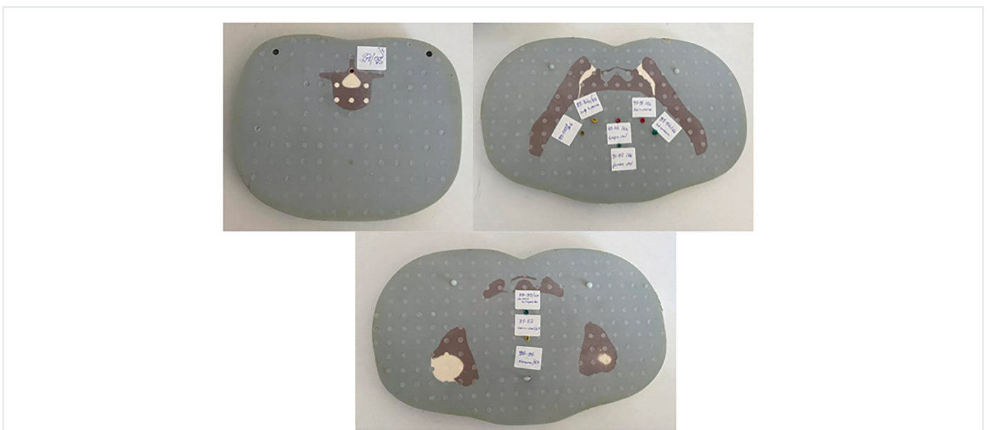
Figure 2. Dosimeters were inserted into cavities corresponding to the ovaries, uterus, and urinary bladder to measure absorbed doses during abdominal CT examinations. CT: Computed tomography
