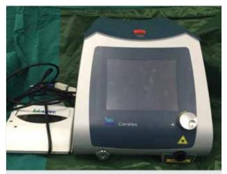
Figure 1. Diode laser (30 W, 980 nm) (Biolitec Ceralas, Bonn, Germany)
